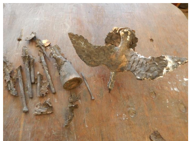
Sculpture after removing the sprue system
