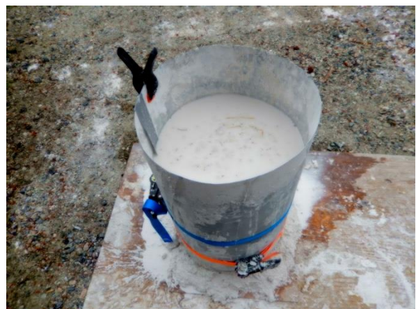
The form filled with grog, plaster, Ludo mass
