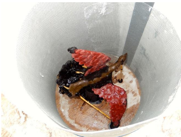
The wax model in the metal form
