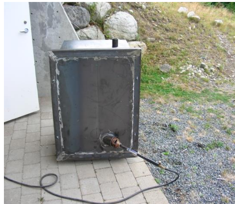
The kiln with a torch
