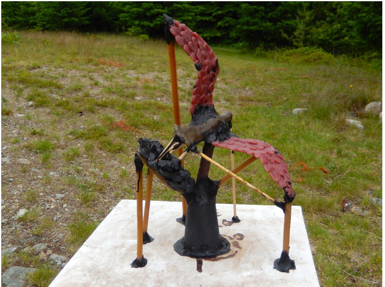
Casting cup/ sprue gate, vents and supports mounted (casting cup shown upside down)
